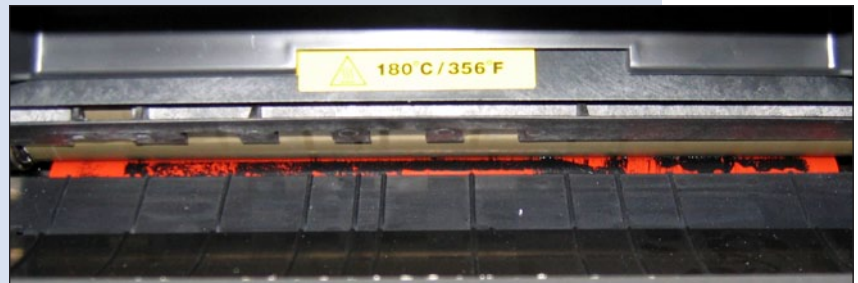
PHOTO 2: Toner buildup on printer fuser back-up roller
