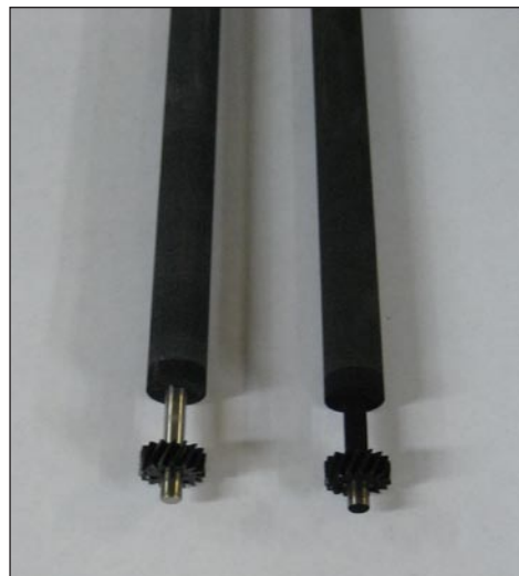
Transfer Roller on Right Shows Excessive Toner Contamination from Brand A Cartridge
